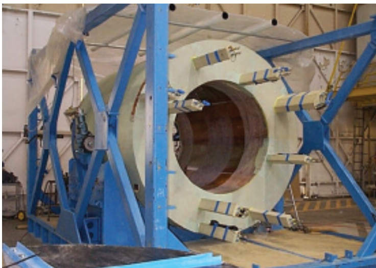
The central solenoid model coil (left), the most powerful pulsed superconducting magnet ever built, plays an essential role in the ITER tokamak fusion reactor (right) now under construction in Cadarache, France.
